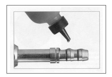
Step 4. Insert the nipple into the hose. To ensure that the nipple is fully inserted, check the gap between the cut end of the hose and the shoulder on the nipple. Care should be taken to avoid kinking or other damage to the hose during nipple insertion.
