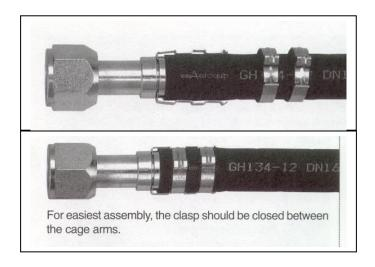
Step 7. Use the pliers to close the clips. The pliers should be positioned squarely on the clip connection points and should remain square during the closing of the clip.
